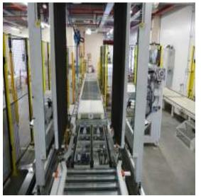
The loading and unloading of the pallet is made by pallet jack, forklift or conveyors when installed in a logistic system. Master Inverter can become part of a logistic system with conveyors and automatic pallet stackers, for non-stop working cycles up to 40 pallets / hour.
