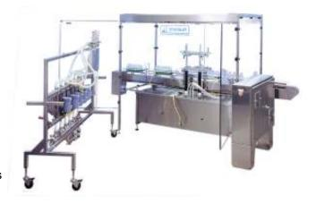
systems that allows you to changeover in less than five minutes. A simple fluid pathway allows for CIP (Clean In Place) or remote CIP.
