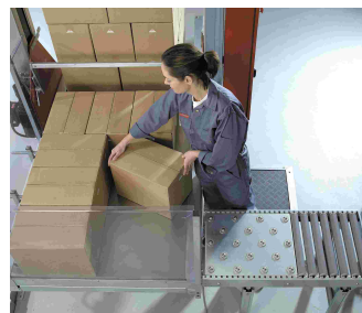
On the stripper plate, the operator forms the desired pattern.
